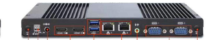
Antenna Hole Extended Power Switch DC-in HDMI 2.0 x 2 USB 3.0 x 2 LAN x 2 Line-out COM port x 2 Antenna Hole
