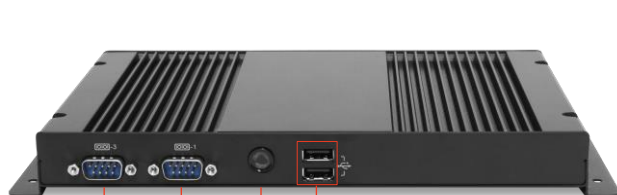
COM3 RS232 x1 COM1 RS232/422/485 x 1 Power Button USB2.0 x 2
